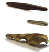
**Step 1.** Use a **center punch**, a pointed tool which dings a small indent in the metal. Line it up with your mark and hit it with a hammer.
